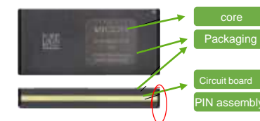
Generation III microchip-500W-1040W/in 3 ChiP4623 (47.91 × 22.8 × 7.21 mm)
